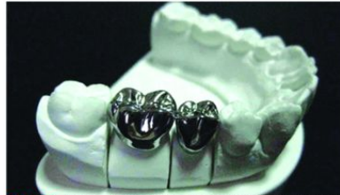
DMLS Direct Metal Laser Sintering Crown with Ceramic Build up DMLS Full Metal
